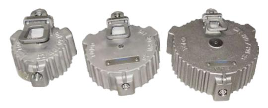
Designed to enhance operator safety & containment security in chemical & gas transport. Pressure indicator, depressurization, customs / tamper seal feature, automatic locking, certified closure. Manually lockable (with padlock). WP: PN 25. Sizes: 2" - 4" and 2" gas adapter.
